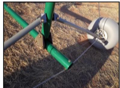
of the trike, look straight down directly above the main cable. The wheel axel should be parallel to the main cable. If not, loosen the aluminum clamp collar to set the axel adjustments. Once the clamp collar is loose, rotate the wheel axel so that it is parallel with the main cable, and retighten the clamp collar. Recheck that the wheel axel is parallel to the main cable and repeat alignment procedure until wheels are aligned. See diagram below.
