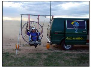
**WARNING:** We do not recommend to run the motor on the trike while it is being hang tested. The torque and thrust forces could create an emergency situation very quickly. If you do want to run up the motor in the hang test rig, you do so at your own risk.
