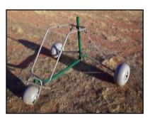
axels, use a rubber mallet to lightly tap the wheel into place. Next, secure the wheel with a clevis pin and ring in the outer hole.
